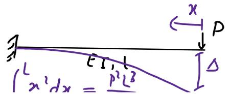
$$W_{int} = U = \frac{1}{2} \int_0^L \frac{M^2}{EI} dx = \frac{1}{2} \int_0^L \frac{(-Px)^2}{EI} dx = \frac{P^2}{2EI} \int_0^L x^2 dx = \frac{P^2 L^3}{6EI}$$
