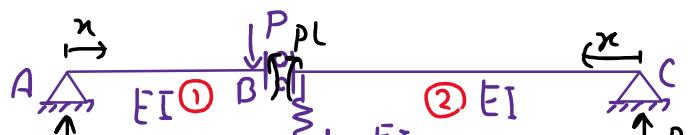
$$\delta_{BL} = \int \frac{M}{EI} \left( \frac{\partial M}{\partial P} \right) dx + \frac{F}{K} \left( \frac{\partial F}{\partial P} \right)$$
