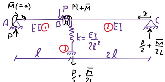
$$\theta_A = \frac{1}{EI} \int_0^L (Px)(1) dx + \frac{1}{EI} \int_0^{2L} \left(\frac{P}{2}x\right)\left(\frac{x}{2L}\right) dx + \frac{\frac{P}{2}}{\frac{EI}{2L^3}} \left(\frac{1}{2L}\right)$$
