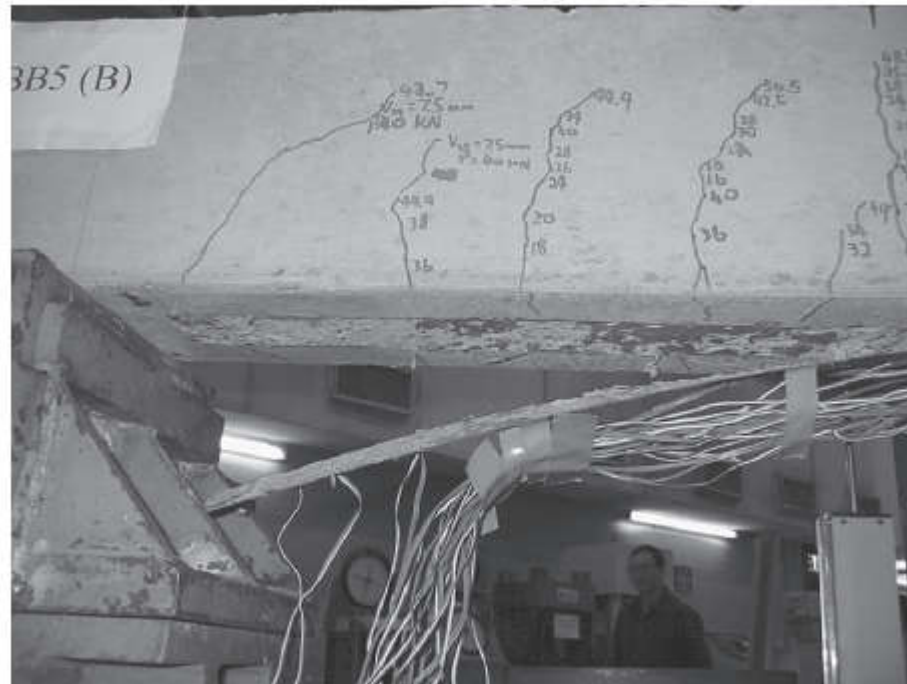
4.8 FRP-plated RC beam: plate-end interfacial debonding.
