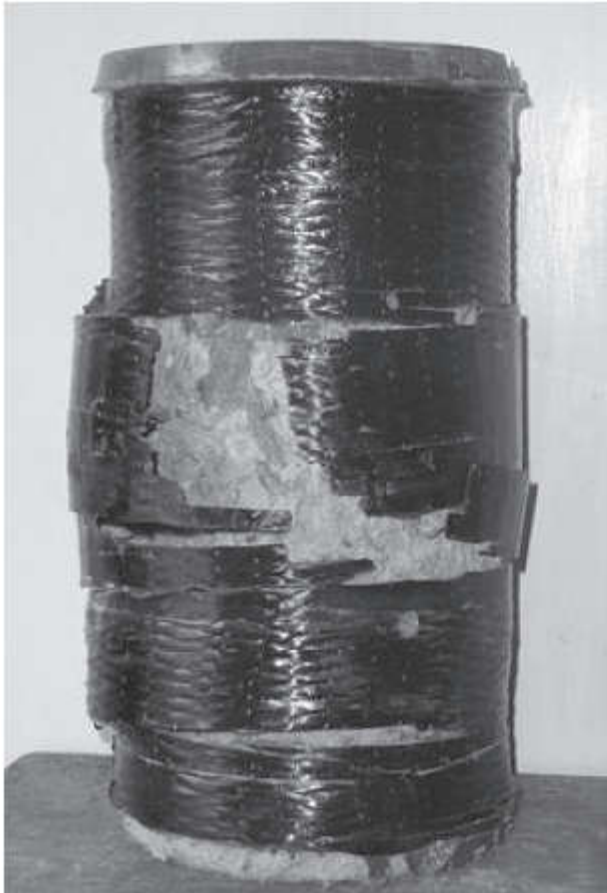
6.2 Failure of an FRP-confined circular concrete column by FRP rupture.
